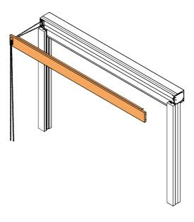
c) Operate the screen fully to ensure the ball chain joiner won't become lodged in the top guide. If it does, pull screen tube out and reposition the ball chain and the sprocket.
