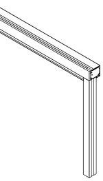
a) A ball chain guide may be installed lower than 1600mm above floor level if the ball chain is sufficiently secured or tensioned to prevent a loop 220mm or longer from
