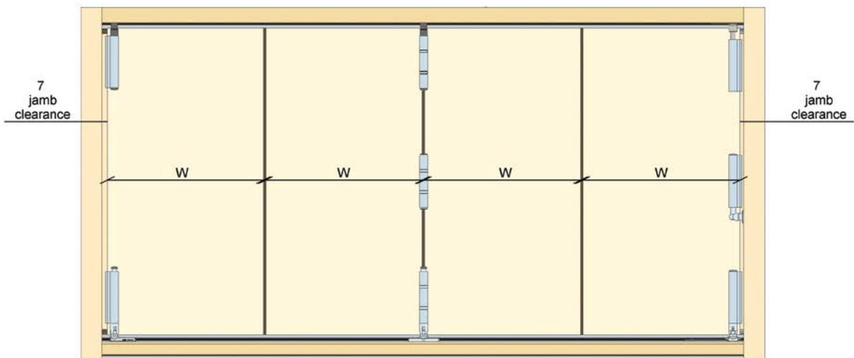
Note: On even panel configurations where a left and right carrier meet (e.g. 2L/2R, 4L/2R) the gap between the panels will be 8mm, and will therefore need weatherseals on both panels.
