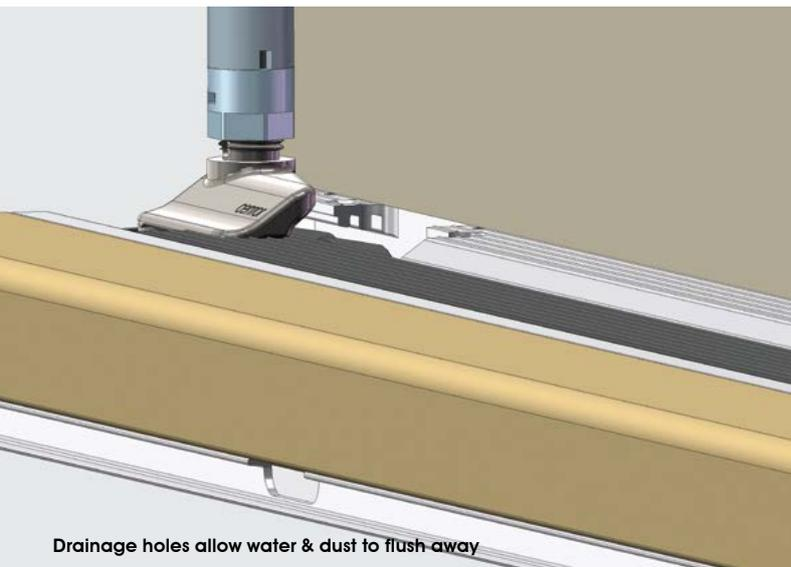
Drainage holes allow water & dust to flush away
