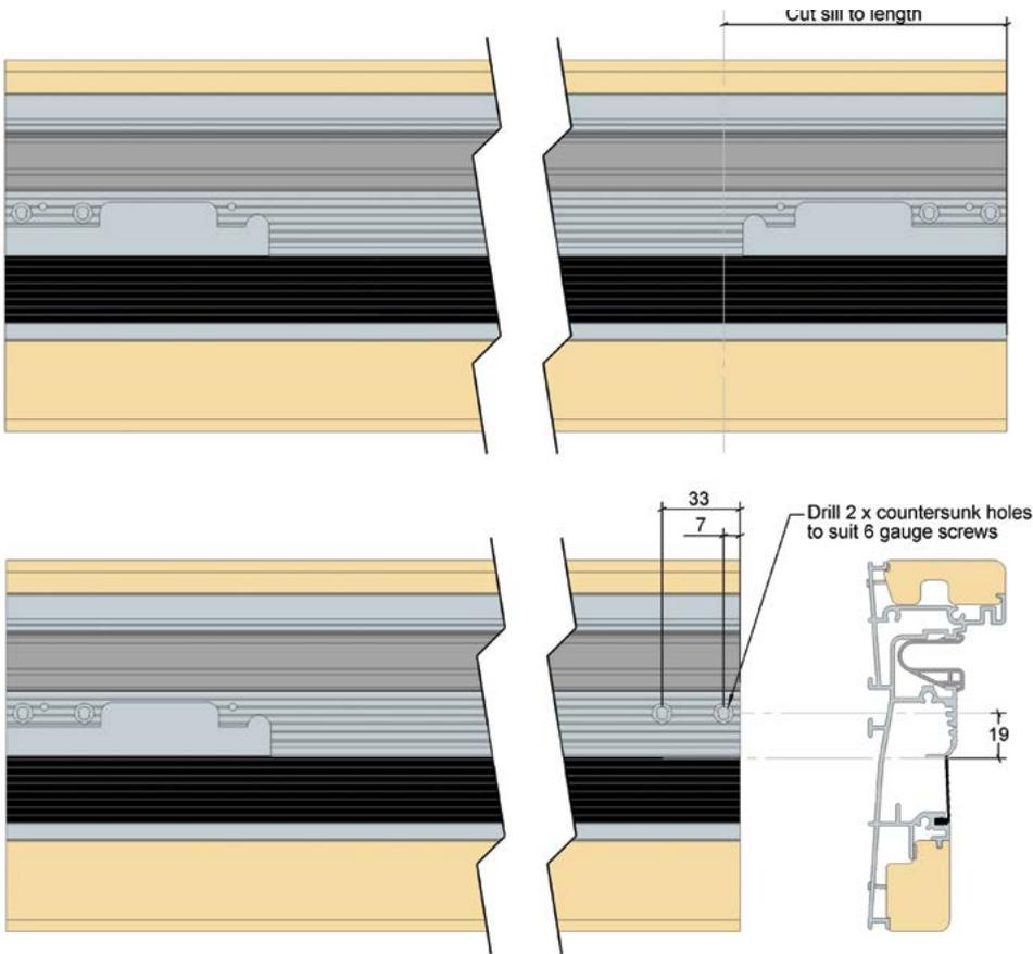
All sills are provided 130mm longer than required, with pivot cutouts at both ends. For single-ended configurations that do not require a second pivot cutout, cut off the non-pivot end to suit the opening size. For double-ended configurations, remove either end when cutting the sill to suit the opening size. To fix off the pivot block, drill two holes as shown. When installing the hardware, feed in the pivot end without the cutout first.
