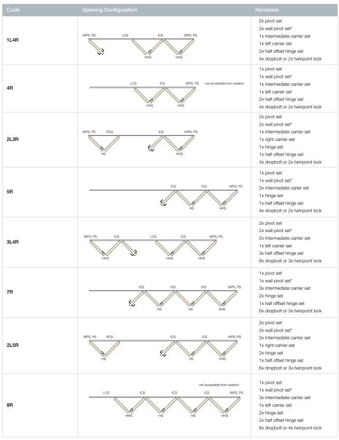
\*Wall Pivot Set required for doors over 2250mm
