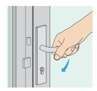
2. Unlock the door by pushing the handle downwards. This retracts the auxiliary bolts and also retracts the door latch.
