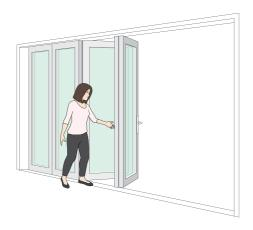
Close the next set of folding door pairs, using the recessed handle on the edge of the door to pull them closed.
