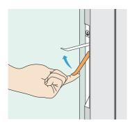
If you have a keyed AutoLatch™, then additionally you can key lock the doors. The key cylinder is concealed in the edge of the stile near the glass, and the locking operation is a 45° turn of the key which creates a distinct click, and when locked the lever can no longer be operated.
