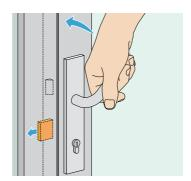
Lock the mechanism by rotating the key through 360°. (Note the key will only turn in one direction). When locked, the lever can no longer be operated from either inside or outside – check this by attempting to open the door.
