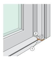
Autolatch™ bolts at the top and bottom of locking locations. These are located at the top and bottom of the panels which house the hidden handle.
