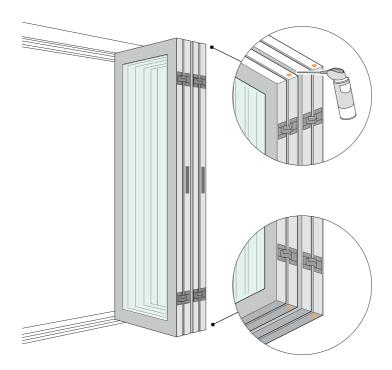
6. Door handles and key cylinders. Use a PTFE based dry lubricant spray. Teflon by DuPont® is one well-known trademark for PTFE. For key cylinders, use an extension nozzle, spray lightly into the keyway, then insert and remove the key 10 times to disperse the lubricant inside the cylinder before it dries.
