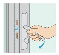
It is recommended that the auxiliary bolts are engaged when the doors are closed.
