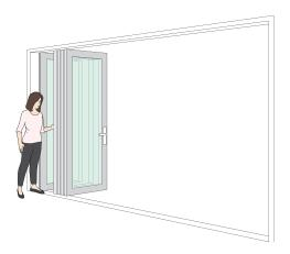
Gently push on the stacked panels while ensuring the access panel is folded flat against the nearest panel.
