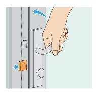
Lock the mechanism by rotating the thumbturn or key through 360°. (Note the thumbturn or key will only turn in one direction). When locked, the lever can no longer be operated from either inside or outside – check this by attempting to open the door.
