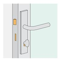
7. Key cylinders. Use a PTFE based dry lubricant spray. Teflon by DuPont® is one well-known trademark for PTFE. Using an extension nozzle, spray lightly into the keyway, then insert and remove the key 10 times to disperse the lubricant inside the cylinder before it dries.
