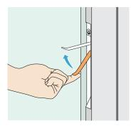
If you have a keyed Centor AutoLatch™, then additionally you can key lock the door or window. The key cylinder is concealed in the edge of the stile near the glass, and the locking operation is a 45° turn of the key which creates a distinct click, and when locked the lever can no longer be operated.
