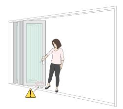
If you use the access panel to pull the doors closed, the outside edge of the access panel could drag along the ground causing damage to both the floor and doors.
