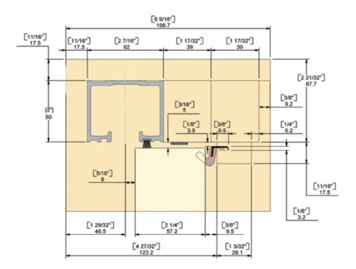
E3 Header for 2-1/4" (57.2mm) door thickness
