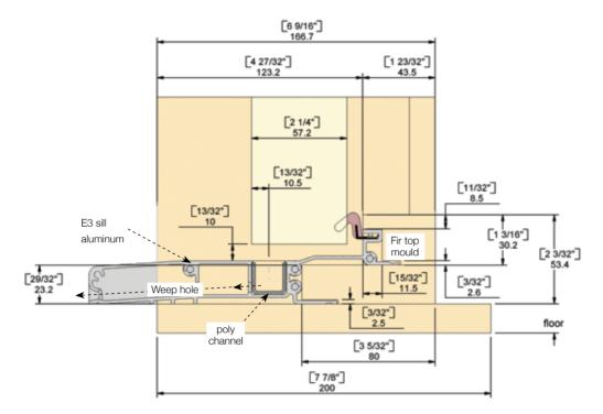
E3 Sill System for 1-3/4" (44.5mm) door thickness
