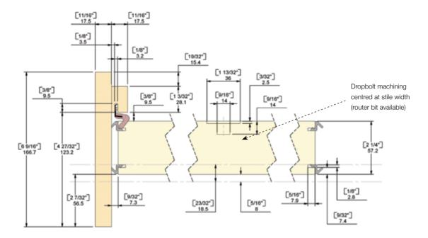
E3 Jamb for 1-3/4" (44.5mm) door thickness
