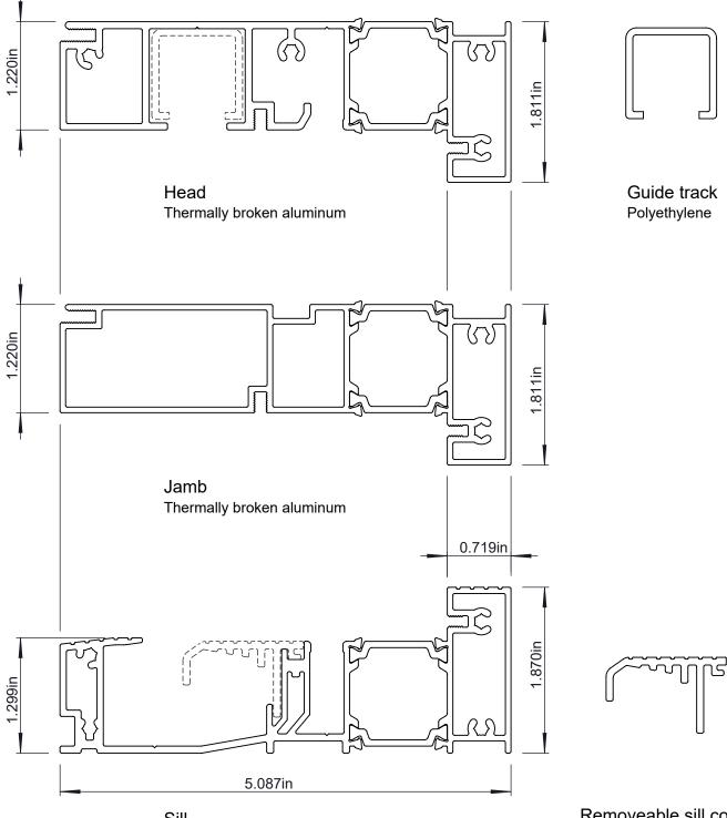
Sill Thermally broken aluminum
