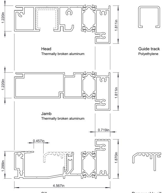
Sill Thermally broken aluminum
